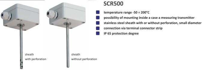
Resistance thermometers SCR500 are designed for ambient temperature measurement. There is a possibility of assembling a programmable temperature transmitter with a 4...20 mA output signal into the housing. The protection tube with perforation allows for quick and precise temperature measurement, thanks to direct contact of thermometric resistor with ambient temperature.
