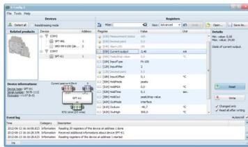
**S-Config 2** is used for the simultaneous detection of devices in multiple Modbus RTU networks and allows user to change the configuration of most of them. For each detected device a list of its registers, which the user can modify, is displayed and also additional informations about device parameters (type, address in the network, etc.).
