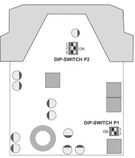
The input and output standard settings are made by setting the code switch levers (one set of switches on the input terminal side and one set of switches on the output terminal side) according the table below.
