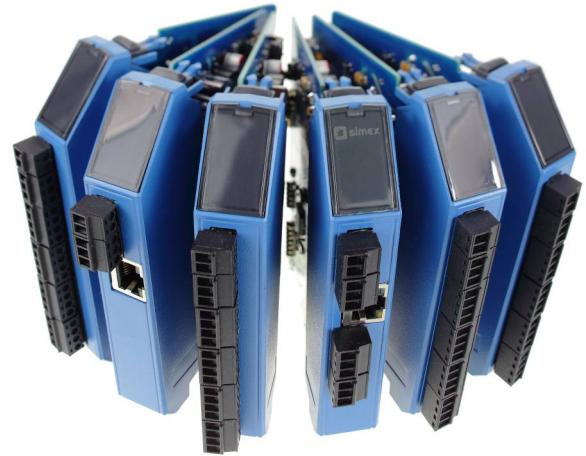
Do you need a measurement and control device for a specific task? Dear User, evaluate the complexity of the application and the number of inputs and outputs. Select a base card, add appropriate I/O cards, insert a communication card with the web server. Upload the logical configuration (and here the free SimFlexSoft configurator will be invaluable) and you're done...
