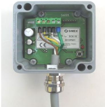
Figure 4.4. Properly made connection
