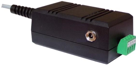
The **SRS-2/4-Z45** converter module is designed to interconnect MASTER devices equipped with RS-232 to RS-485 bus. The module can work either with devices controlling direction of transmission (via RTS line), or devices not controlling the direction (control is then fully automatic). The MASTER functions can be realized by any device, e.g. PC computer with dedicated software. Connection of more than one MASTER device to the RS-485 bus is prohibited.
