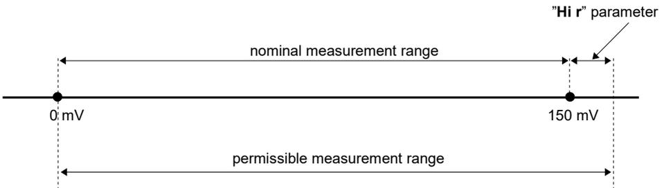
Figure 6.2. Definitions of measurement ranges in mode 0 ÷ 150mV
