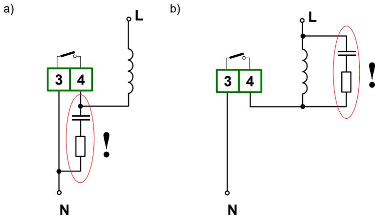
Figure 4.15. Examples of suppression circuit connection:
