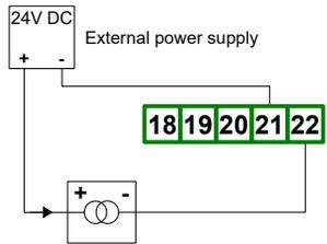
Figure 4.10. Connection of 2-wire current converters
