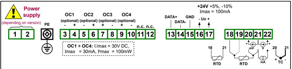
Figure 4.6. Terminals description (four OC-type outputs)
