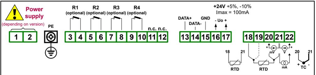
Figure 4.5. Terminals description (four relay outputs)
