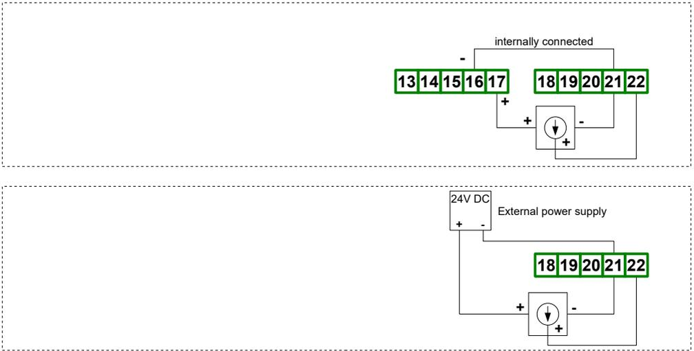
Figure 4.12. Connection of voltage converters
