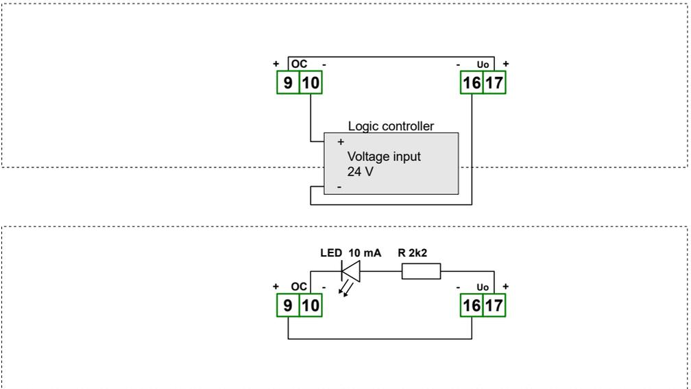
Figure 4.16. Example of OC-type outputs connection
