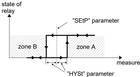
Figure 6.5. One threshold control of the relay outputs
