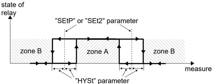
Figure 6.6. Two threshold control of the relay outputs
