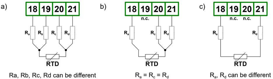
Figure 4.13. Connection of RTD sensors:
