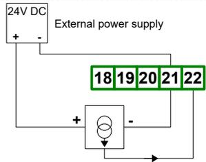
Figure 4.11. Connection of 3-wire current converters
