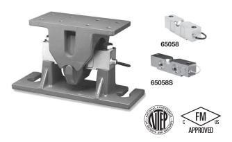
This product is designed to simplify the installation of the 65058 load cell into a certified Legal-for-Trade high capacity weigh bridge. Unilink™ floating suspension allows controlled floating of the scale deck, providing a reliable and accurate weighing system. The load cell is nickel plated or stainless steel and sealed to IP67 standards, assuring reliability. The mount assembly is provided with a primer coat finish to simplify the manufacture of the scale.
