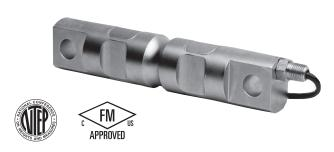
This product is designed for use in industrial and out-door environments. Nickel plated steel construction limits corrosion from outdoor use. The IP67 sealing makes it suitable for applications that are subject to high-pressure wash down. Tank weighing is made simple when this load cell is combined with the EZ mount mounting hardware it was designed for. Its high accuracy and availability in high capacities make it ideal for certified truck and rail scales.
