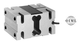
A special humidity resistant protective coating assures long-term reliability. The two additional sense wires feed back the voltage reaching the load cell. Complete compensation of changes in lead resistance, due to temperature change and/or cable extension, is achieved by feeding this voltage into the appropriate electronics.
