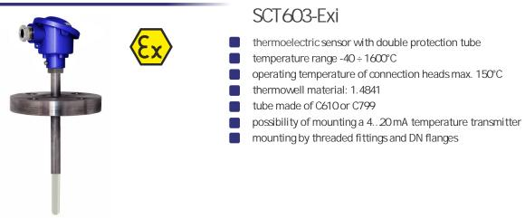
The thermocouple SCT603-Exi is intended for measuring the temperature of pipelines, tanks and boilers. The sensor is designed to work in difficult conditions (gases, vapors) and high temperatures up to 1600°C. The sensor consists of an aluminum connection head, a steel transition cover and a ceramic cover. The sensor is made with a replaceable measuring insert, which makes it possible to regenerate the element without having to dismantle the entire cover.
