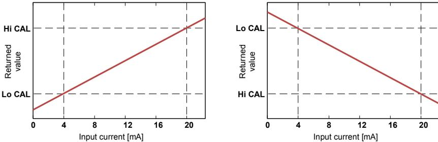
Figure. 6.1 Normal („Lo CAL” < ”Hi CAL”) and inverted („Lo CAL” > ”Hi CAL”) characteristic
