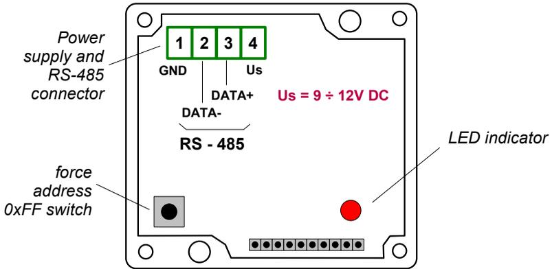
Figure 4.3. Location of elements inside the module case
