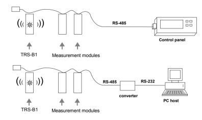
RS-485 bus should be equipped with termination resistors (100-150 ohm) on both ends. The bus must not be ramified, and longer than 1 km.
