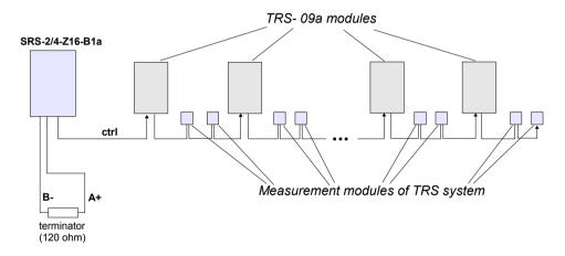
Figure 4.6. Cascade of power supply modules TRS-09a.
