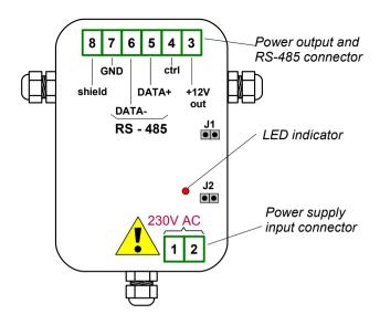
Figure 4.3. Location of elements inside the module case
