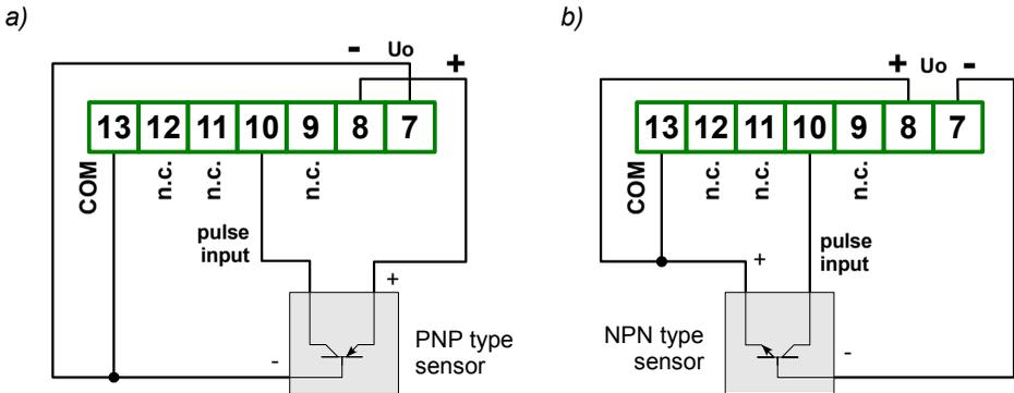
Figure 4.14. An example of sensor connection:
