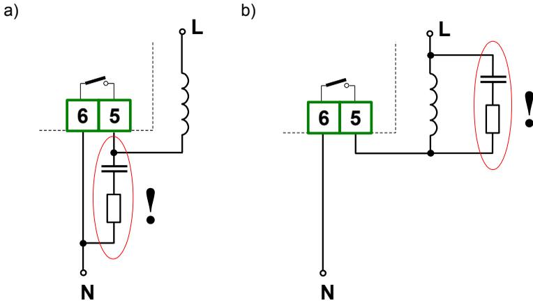
Figure 4.13. Examples of suppression circuit connection:
