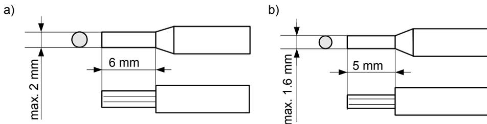
Figure 4.2. Recommended dimensions of cable stripping
