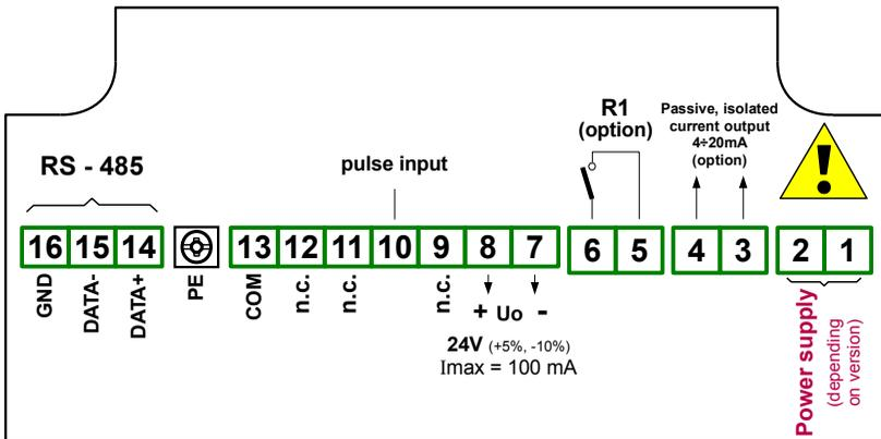
Figure 4.7. Terminals description (relay and passive current outputs)
