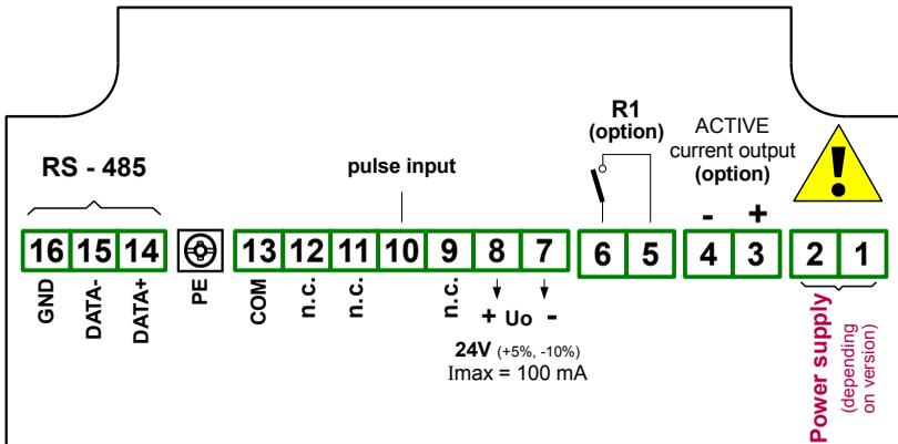
Figure 4.6. Terminals description (relay and active current outputs)
