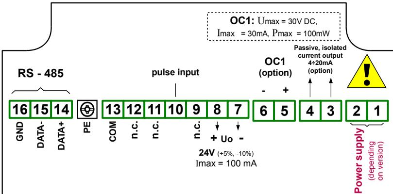
Figure 4.10. Terminals description (OC-type and passive current outputs)
