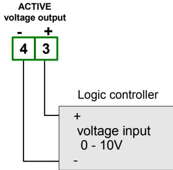
Figure 4.18. Example of active voltage outputs connection
