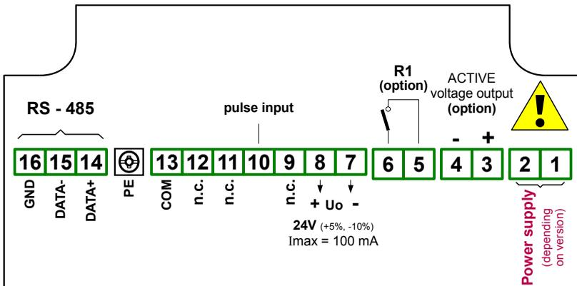
Figure 4.8. Terminals description (relay and active voltage outputs)
