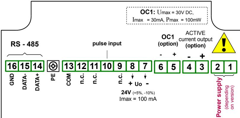
Figure 4.9. Terminals description (OC-type and active current outputs)
