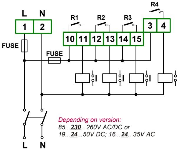
Figure 4.14. Connection of power supply and relays
