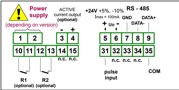
Figure 4.8. Terminals description (relay and active current outputs)
