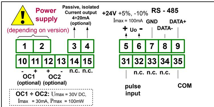
Figure 4.12. Terminals description (OC-type and passive current outputs)
