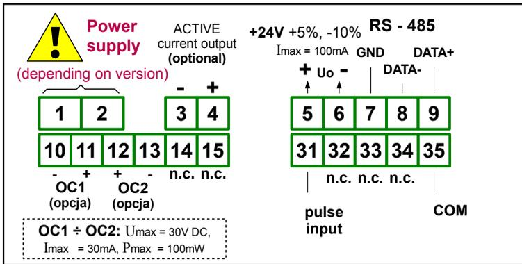
Figure 4.11. Terminals description (OC-type and active current outputs)
