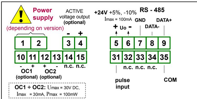
Figure 4.13. Terminals description (OC-type and active voltage outputs)
