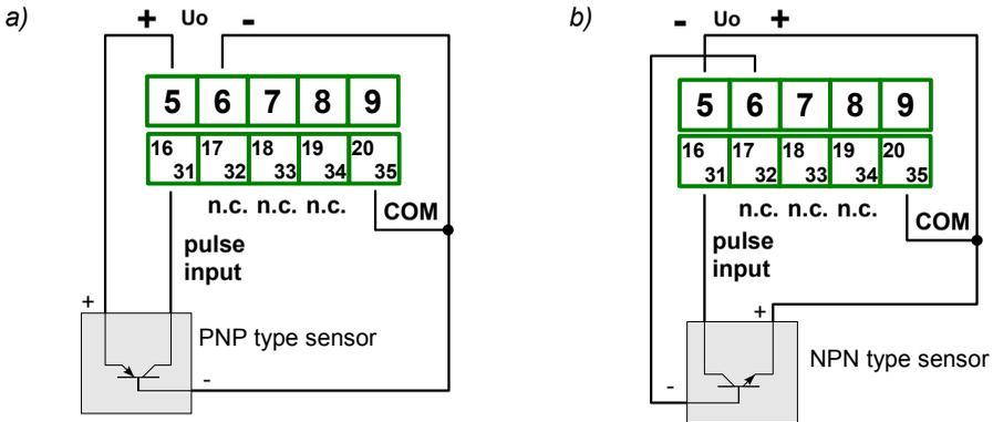
Rys. 4.16. An example of sensor connection:
