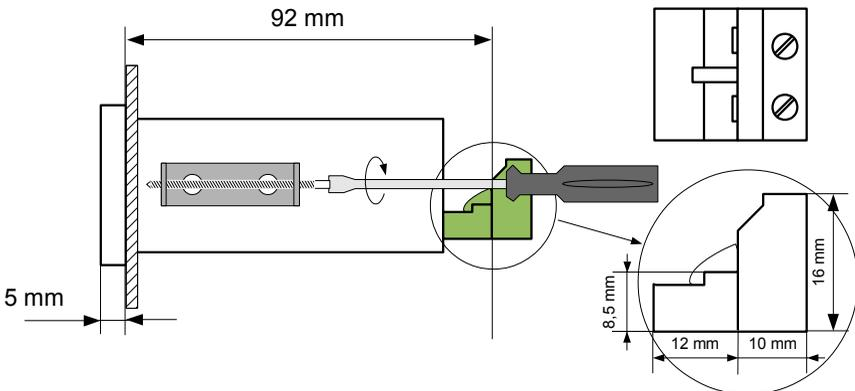
Figure 4.3. Installing of brackets, and dimensions of connectors.
