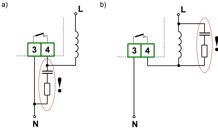
Figure 4.15. Examples of suppression circuit connection:
