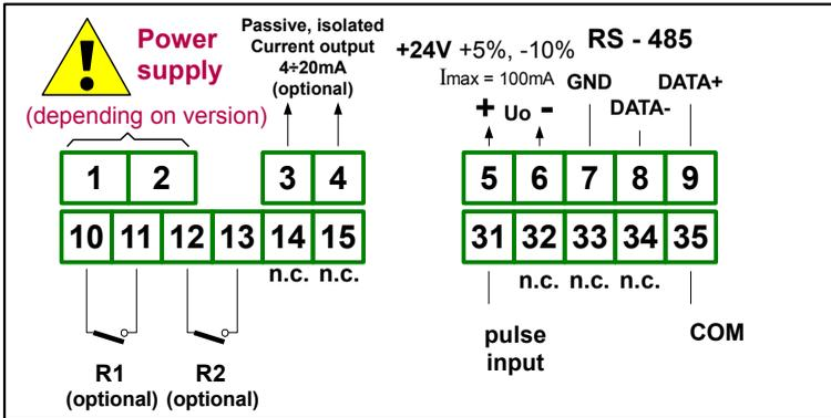
Figure 4.9. Terminals description (relay and passive current outputs)
