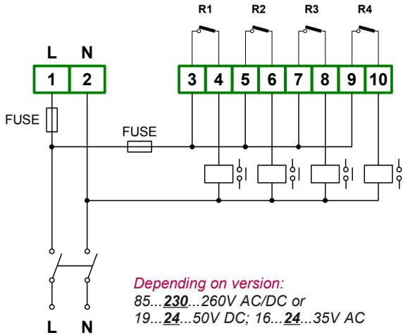
Figure 4.11. Connection of power supply and relays
