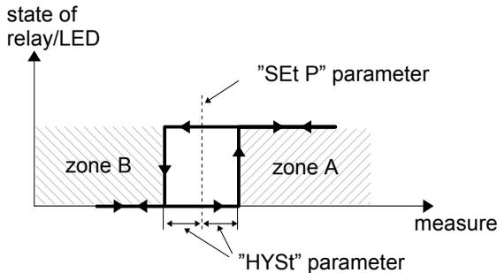
Figure 6.2. One threshold control of the relay/LED outputs
