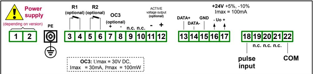
Figure 4.8. Terminals description (two relay, one OC-type and one passive voltage outputs)
