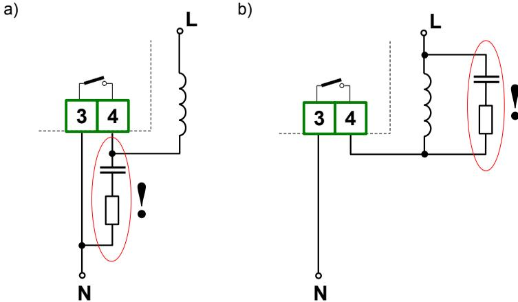
Figure 4.12. Examples of suppression circuit connection:
