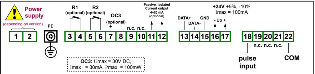
Figure 4.7. Terminals description (two relay, one OC-type and one passive current outputs)
