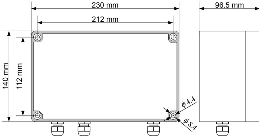
Figure 4.1. Device and assembly dimensions of the case
