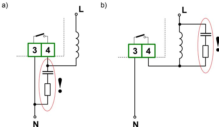
Figure 4.8. Examples of suppression circuit connection:
