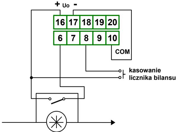
Figure 4.9. Example of connection between flow counter and flow sensor with contactron output
