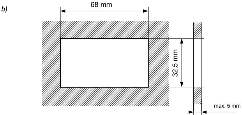
Figure 4.1. Mounting hole dimensions: a) recommended b) allowable
