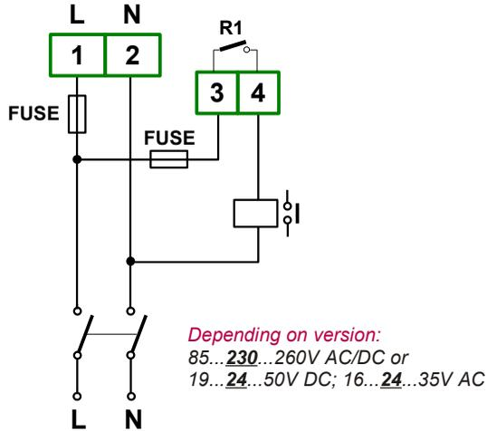
Figure 4.7. Connection of power supply and relays
