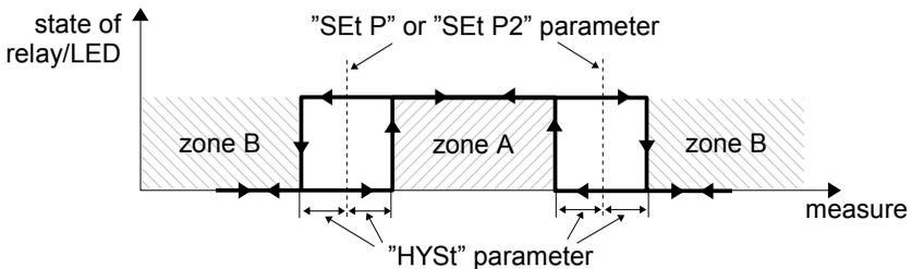
Figure 6.4. Two threshold control of the relay/LED outputs
