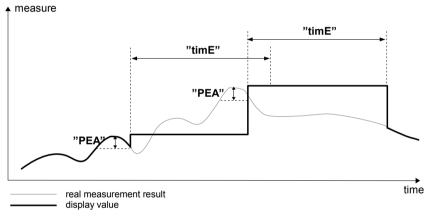
Figure 6.2. Process of peaks detection
