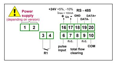
Figure 4.5. Terminals description (relay outputs)
