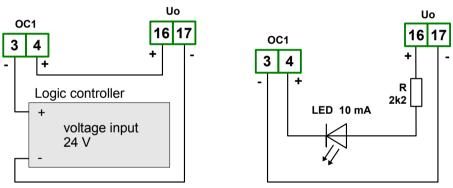
Figure 4.10. Example of OC-type outputs connection
