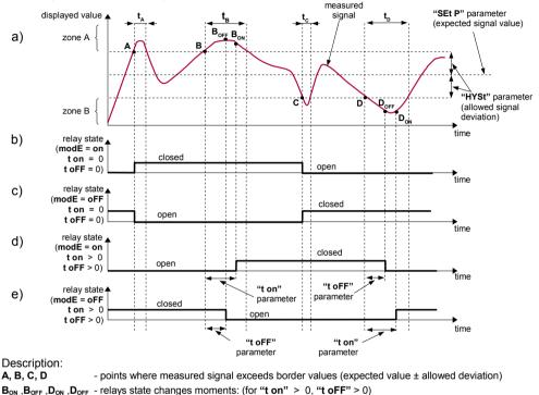
$t_A$ ,  $t_B$ ,  $t_C$ ,  $t_D$  - time periods while input signal is in zone A or zone B
