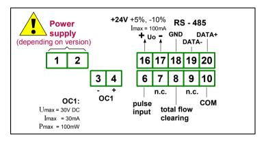
Figure 4.6. Terminals description (OC-type outputs)
