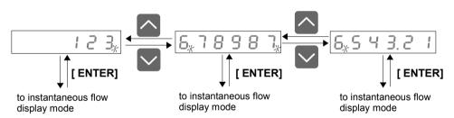
Figure 6.1. Switching between digits (screens) of total flow result.
