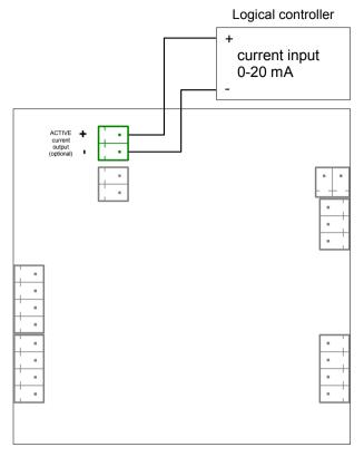
Figure 4.10. Example of active current outputs connection (for device with active current output only)
