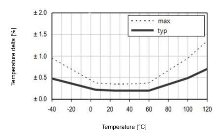
Figure 3.4. Maximal tolerance for temperature for humidity sensor
