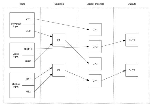
Figure 6.1. General logical structure of block connections
