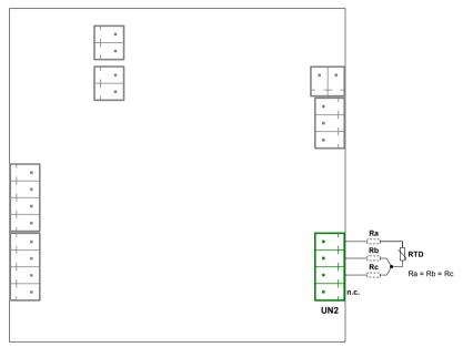
Figure 4.7. Connection of RTD sensors 3-wire circuit
