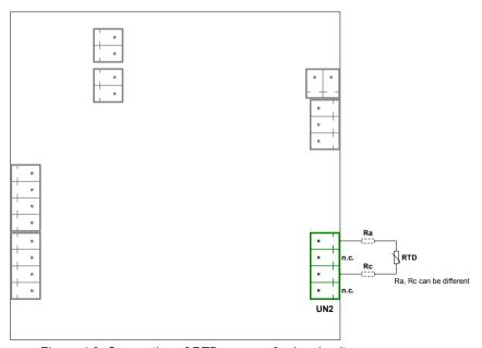
Figure 4.8. Connection of RTD sensors 2-wire circuit
