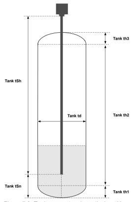
Figure 7.3. Tank parameters in vertical position
