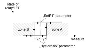
Figure 6.14. One threshold control of the relay/LED outputs
