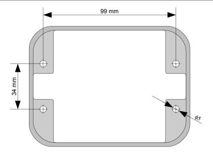
Figure 4.1. Recommended mounting hole dimensions
