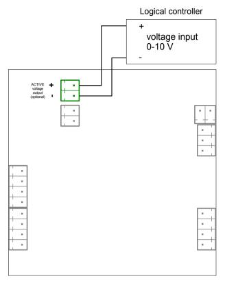
Figure 4.12. Example of active voltage outputs connection (for device with active voltage output only)
