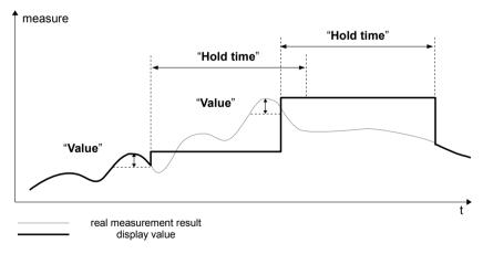
Figure 6.4. Process of peaks detection
