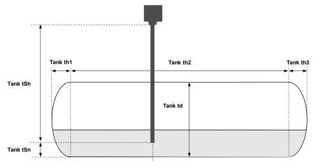
Figure 6.11 Parameters of cylindrical tank in horizontal position.
