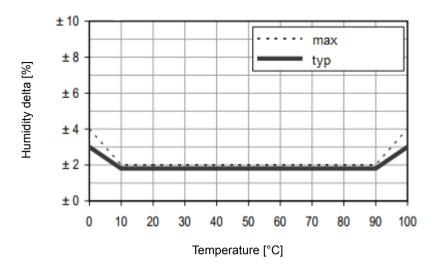
Figure 3.3. Typical and maximal tolerance at 25°C for humidity
