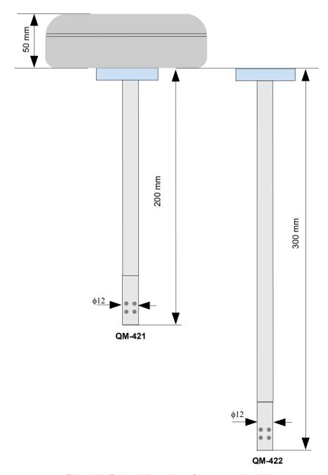
Figure 4.3. External dimensions of sensors series 400
