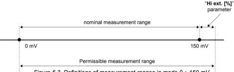
Figure 6.3. Definitions of measurement ranges in mode 0 ÷ 150 mV
