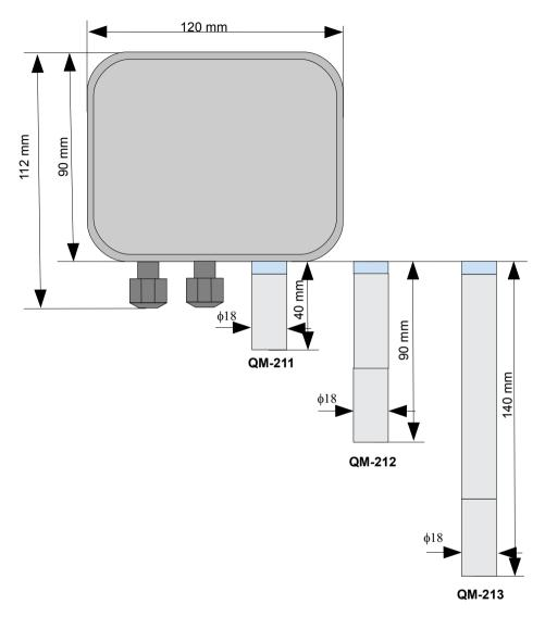
Figure 4.2. External dimensions of sensors series 200
