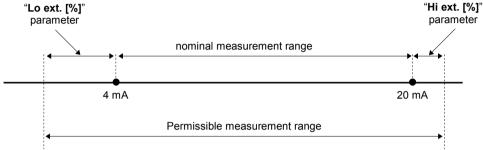
Figure 6.2. Definitions of measurement ranges in mode 4 ÷ 20 mA
