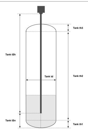
Figure 6.10 Parameters of cylindrical tank in vertical position.
