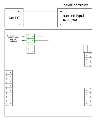
Figure 4.11. Example of passive current outputs connection (for device with passive current output only)
