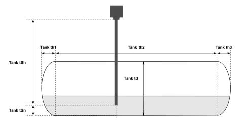
Figure 7.4. Tank parameters in horizontal position
