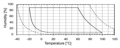
Figure 3.1. Operating conditions for the humidity sensor
