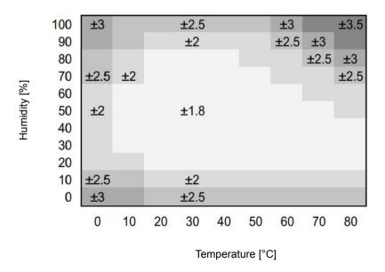
Figure 3.2. Maximal tolerance of humidity measurements given in % RH for the humidity sensor
