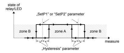
Figure 6.15. Two threshold control of the relay/LED outputs
