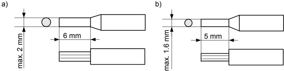
Figure 4.2. Recommended dimensions of cable stripping
