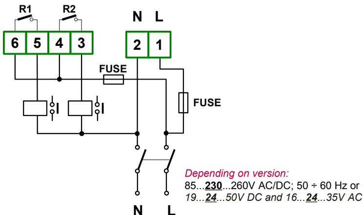
Figure 4.12. Connection of power supply and relays
