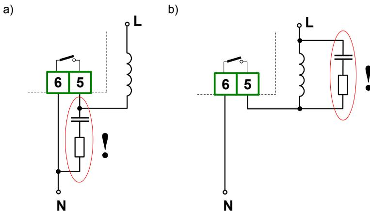
Figure 4.13. Examples of suppression circuit connection:
