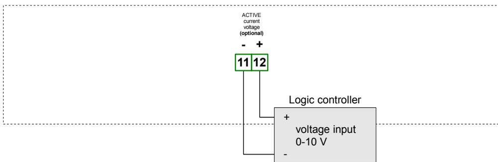
Figure 4.19. Example of active voltage outputs connection
