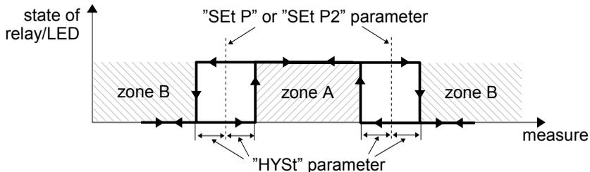
Figure 6.4. Two threshold control of the relay/LED outputs
