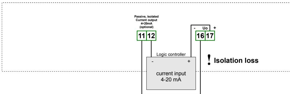
Figure 4.18. Example of passive current outputs connection
