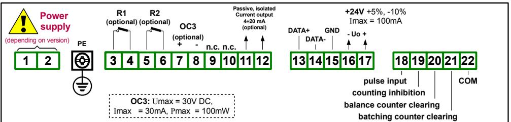
Figure 4.7. Terminals description (two relay, one OC-type and passive current outputs)
