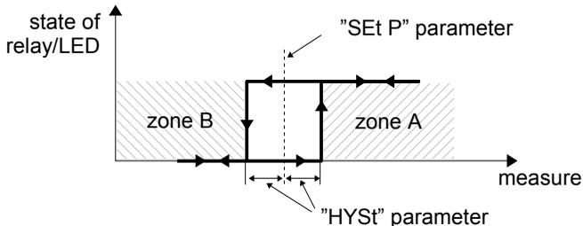
Figure 6.3. One threshold control of the relay/LED outputs
