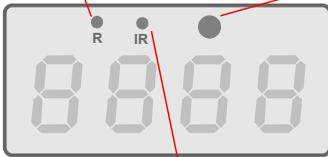
IR LED confirms that the infrared receiver is on
