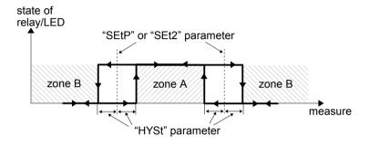
Figure 6.4. Two threshold control of the relay/LED outputs
