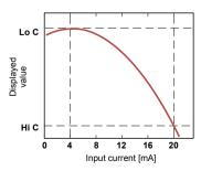
Figure. 9.2 Normal ("Lo C" < "Hi C") and inverted ("Lo C" > "Hi C") characteristic
