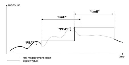
Figure 6.2. Process of peaks detection
