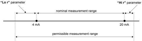
Figure 6.1. Definitions of measurement ranges in mode 4 ÷ 20mA
