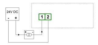
Figure 4.6. Connection of 2-wire current converters
