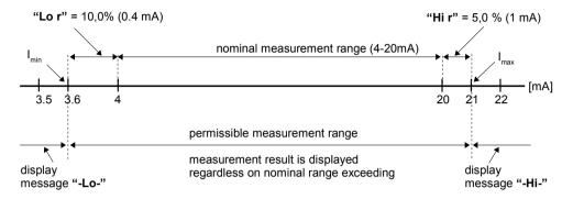
Figure 7.1 Example of definition of permissible range of input signal "Lo r" and "Hi r" parameters
