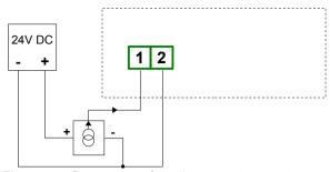
Figure 4.7. Connection of 3-wire current converters
