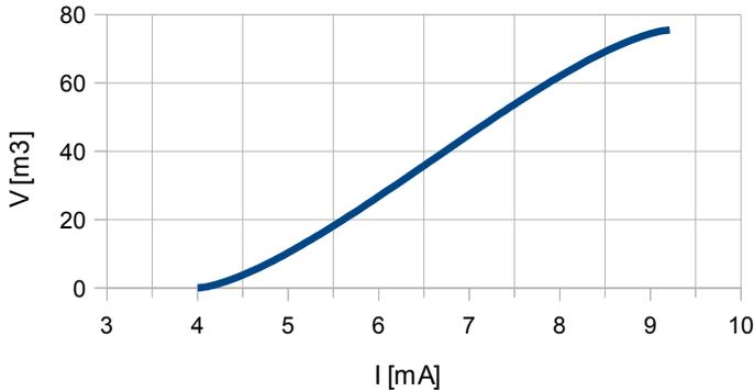
Figure 9.7 The volume characteristic of tank depending on input current in 4÷20mA range.
