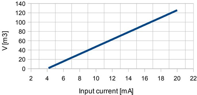
Figure 9.6 The volume characteristic of tank depending on input current in 4÷20mA range.
