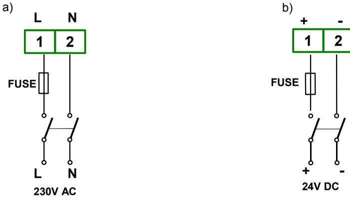
Figure 4.6. Connection of power supply
