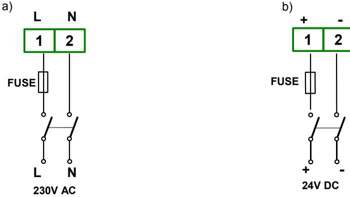
Figure 4.6. Connection of power supply
