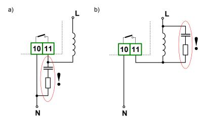
Figure 4.8. Examples of suppression circuit connection: a) to relay terminals; b) to the inductive load
