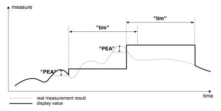
Figure 6.1. Process of peaks detection
