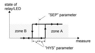
Figure 6.2. One threshold control of the relay/LED output
