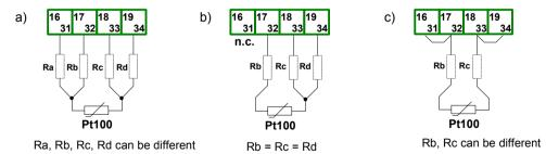
Figure 4.9. Connection of sensors:
