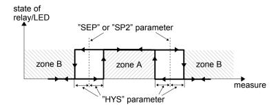
Figure 6.3. Two threshold control of the relay/LED output
