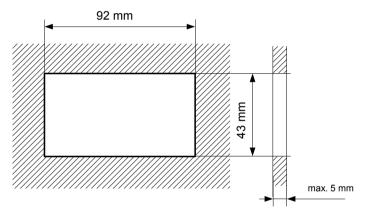
Figure 4.2. Allowable mounting hole dimensions
