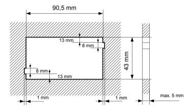
Figure 4.1. Recommended mounting hole dimensions
