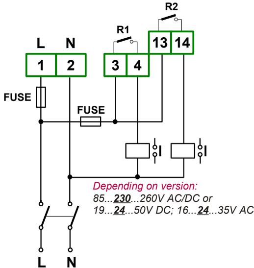
Figure 4.7. Connection of power supply and relays
