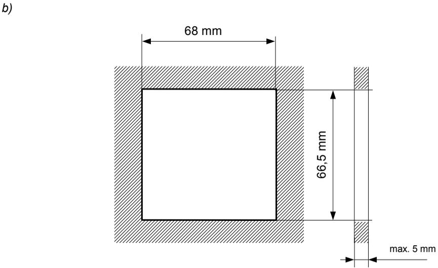
Figure 4.1. Mounting hole dimensions: a) recommended b) allowable
