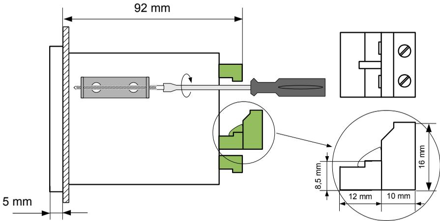
Figure 4.2. Installing of brackets, and dimensions of connectors.
