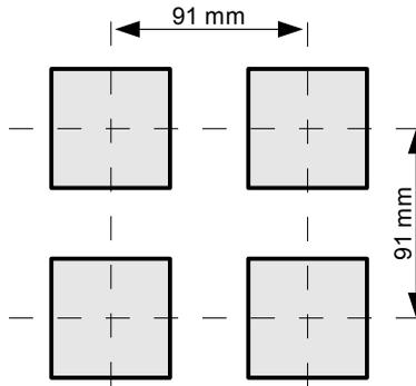
Figure 4.3. Minimum distances when assembly of a number of units
