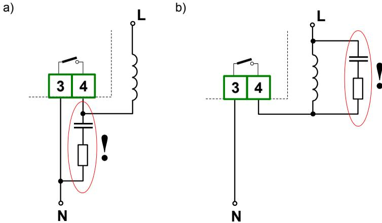
Figure 4.8. Examples of suppression circuit connection:
