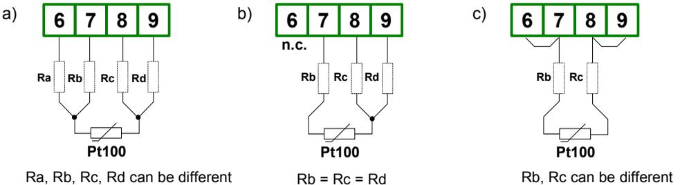
Figure 4.10. Connection of sensors:
