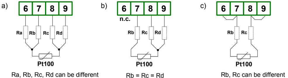
Figure 4.10. Connection of sensors:
