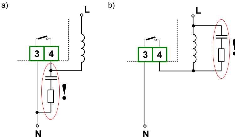
Figure 4.8. Examples of suppression circuit connection:
