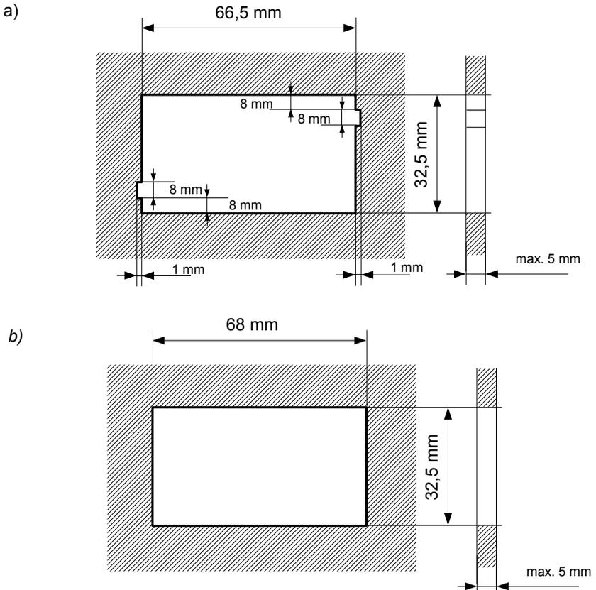
Figure 4.1. Mounting hole dimensions: a) recommended b) allowable
