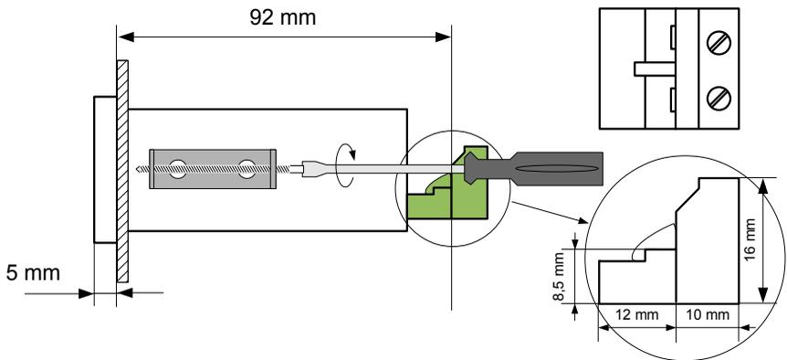
Figure 4.2. Installing of brackets, and dimensions of connectors.
