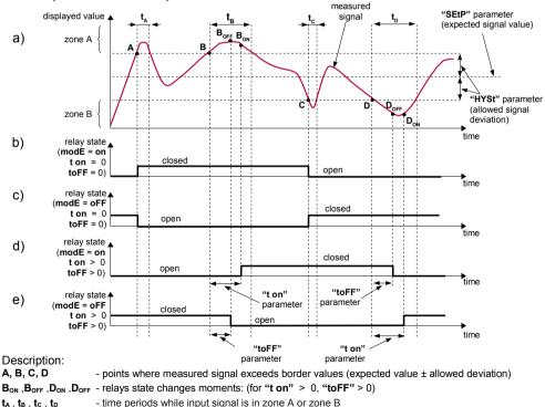
Figure 6.4. Principle of LED/relay output operation for one threshold mode
