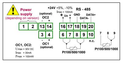
Figure 4.6. Terminals description (OC-type outputs)
