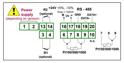
Figure 4.5. Terminals description (relay outputs)
