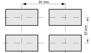
Figure 4.3. Minimum distances when assembly of a number of units
