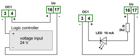
Figure 4.9. Example of OC-type outputs connection
