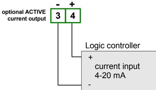
Figure 4.12. Example of current outputs connection
