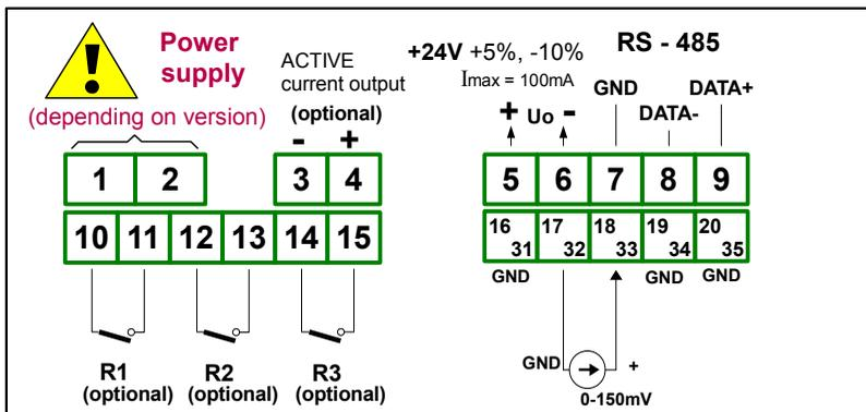
Figure 4.7. Terminals description (relay outputs, device with current output)
