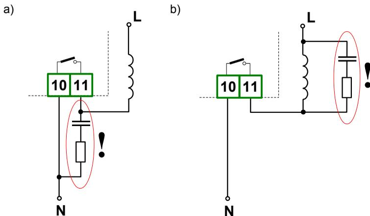
Figure 4.9. Examples of suppression circuit connection:
