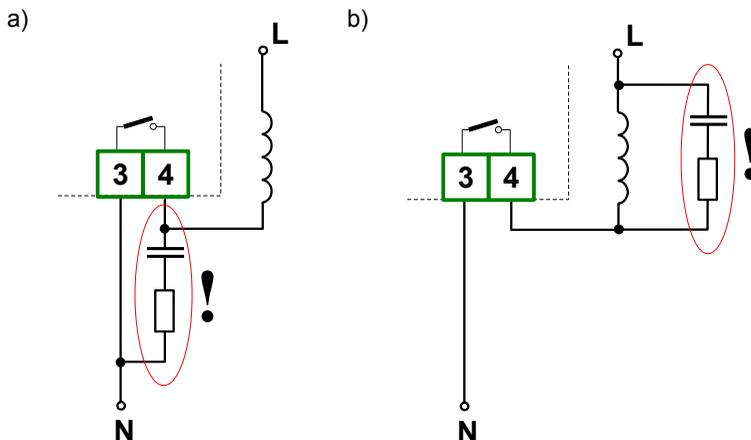
Figure 4.8. Examples of suppression circuit connection:
