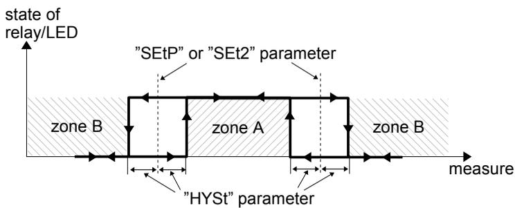
Figure 6.4. Two threshold control of the relay/LED outputs
