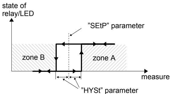
Figure 6.3. One threshold control of the relay/LED outputs
