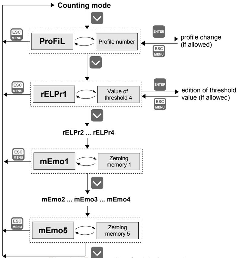
Figure 7.1 Functionality of quick view mode
