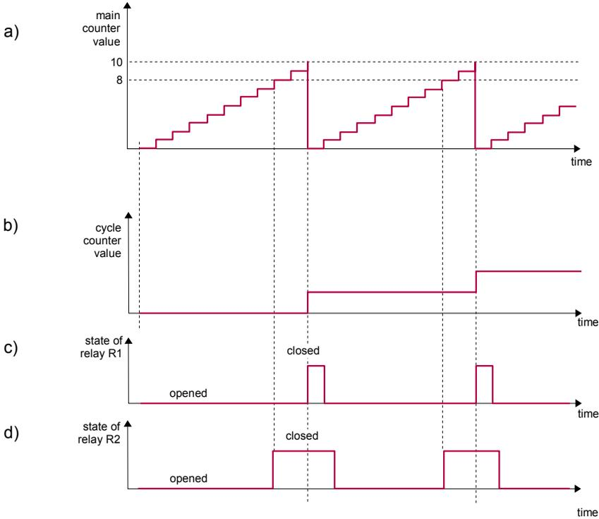
Figure 6.6 Example of relay controlling in „standard” mode;
