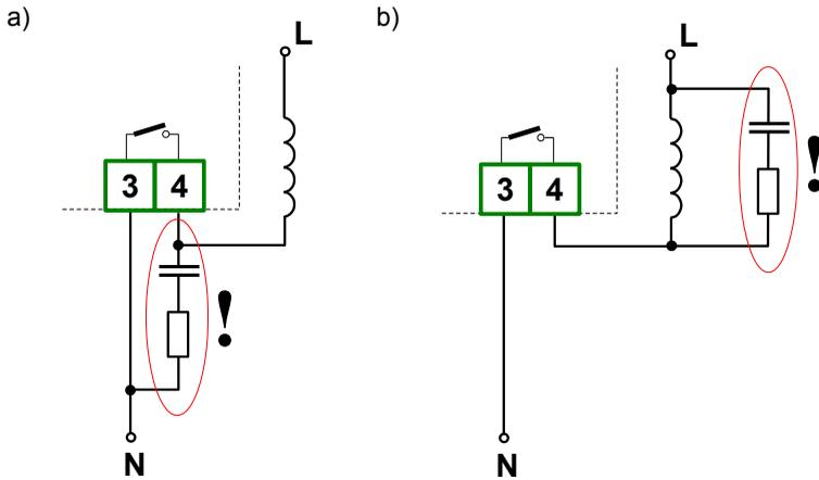
Figure 4.9. Examples of suppression circuit connection:
