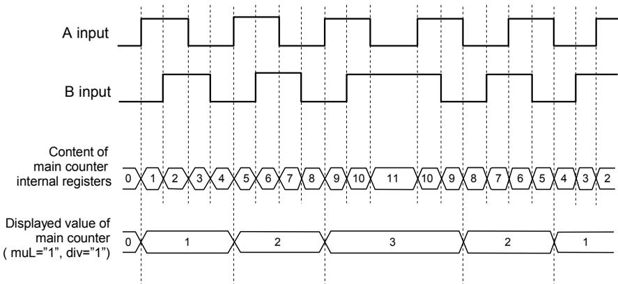
Figure 6.1. The counting principle of the **SLK-94T** counters
