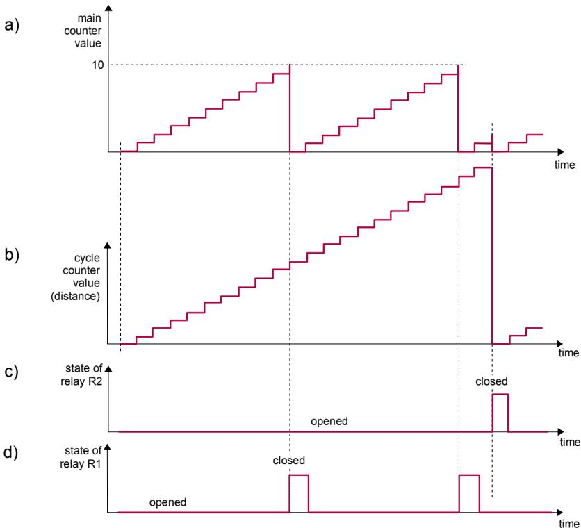
Figure 6.7 Example of relay controlling in „marker” mode;
