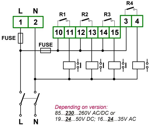
Figure 4.8. Connection of power supply and relays
