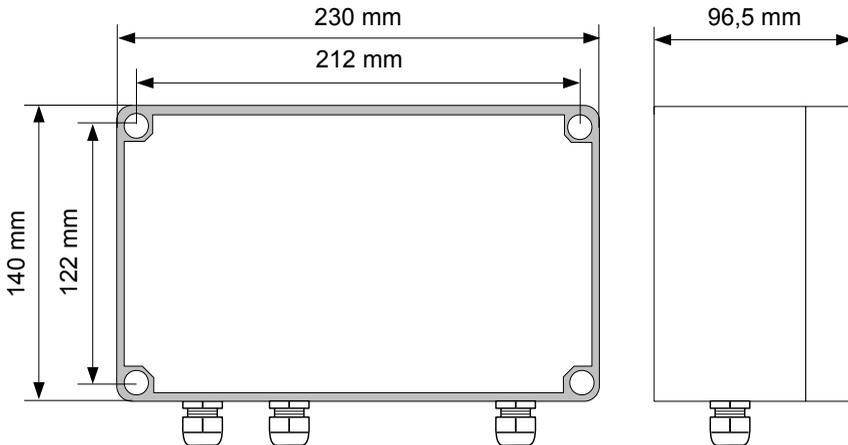
Figure 4.1. Device and assembly dimensions of T-type case
