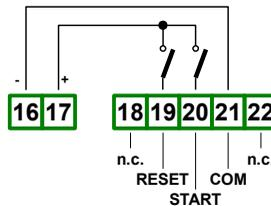
Figure 4.5. Connection of input terminals
