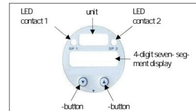
Fig. 3 touchpad for device with two contacts
