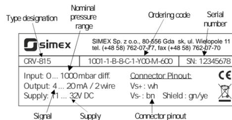
Fig. 1: Manufacturing label- example
