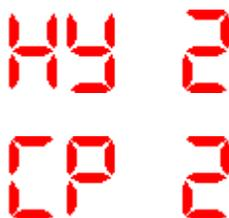
After pressing both the buttons simultaneously, the hysteresis mode and the comparator mode of the switch 2 can be switched. The difference between both the modes of operation is given by the illustration given in the note. Pressing both the buttons simultaneously, the settings are saved.
