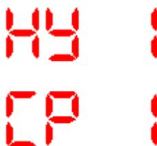
After pressing both the buttons simultaneously, the hysteresis mode and the comparator mode of the switch 1 can be switched. The difference between both the modes of operation is given by the illustration given in the note. Pressing both the buttons simultaneously, the settings are saved.
