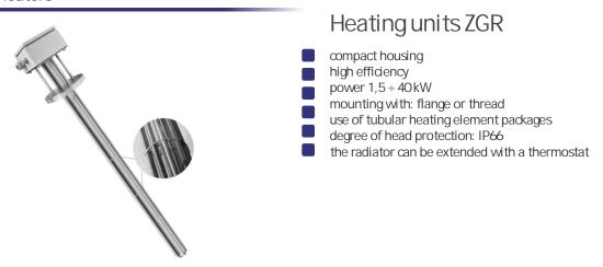
Heating units ZGR type are used for direct heating of a variety of liquids. The compact design makes it possible to put a relatively large power in a single body. The ZGR type heater consists of a package of tubular heating elements soldered into a threaded spigot or flange. An expanded version of the radiator with a thermostat allows you to set the desired temperature of the heated medium without the need for an additional control system.
