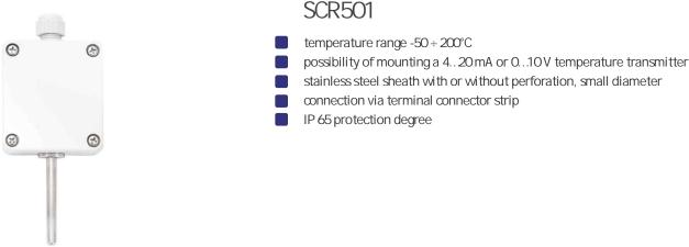
Resistance thermometers SCR500 are designed for ambient temperature measurement inside and outside residential, office and industrial spaces. There is a possibility of assembling a programmable temperature transmitter with a 4...20mA output signal into the housing. The protection tube with perforation allows for quick and precise temperature measurement, thanks to direct contact of thermometric resistor with ambient temperature.
